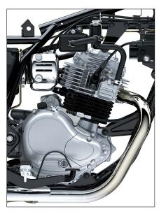
\* The 4-stroke air-cooled single cylinder engine offers both reliability and strong performance, while contributing to a compact package.
