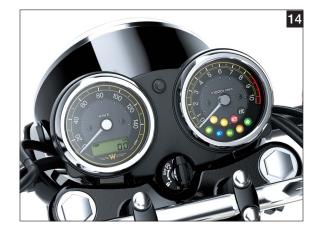
warning lamp, dual turn signal indicators, low fuel level indicator, high beam indicator, and neutral indicator. (Photo 14)
