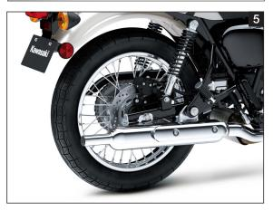
\* The tyres have a profile with a retro style. The tyre sizes are as follows: F: 90/90-18M/C 51S R: 110/90-17M/C 60S ENGINE
